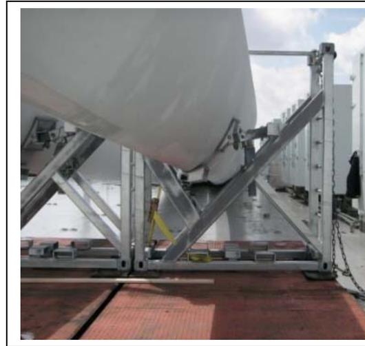
Example of blades shipped individually with a fixed frame on the root and a movable frame placed under the tip. Placement of the cradle along the tip is critical.
