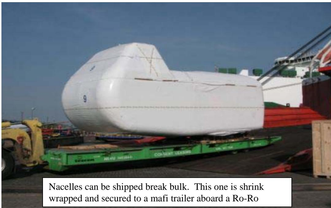
Nacelles can be shipped break bulk. This one is shrink wrapped and secured to a mafi trailer aboard a Ro-Ro
