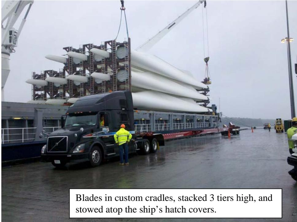
Also deck loading criteria, transport and racking stresses need to be reviewed. The final cradle should have lifting and lashing points clearly marked as well as the center of gravity. Also, the cradle under the blade tip must be placed at a specific distance from the root, to avoid possible deflection of the blade, when lifted or transported. The location of the tip cradle should be marked on the blade.
