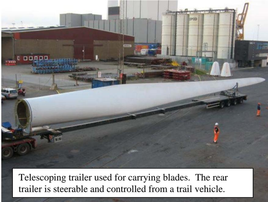
Over the last few years, a 1.5 MW wind turbine has been the prevalent size on U.S. roads and wind farms. It is about the largest and heaviest that transports easily on most U.S. roads. But turbine design is trending to larger units; hence, 2.5 and 3 MW units will soon be more frequently encountered.
