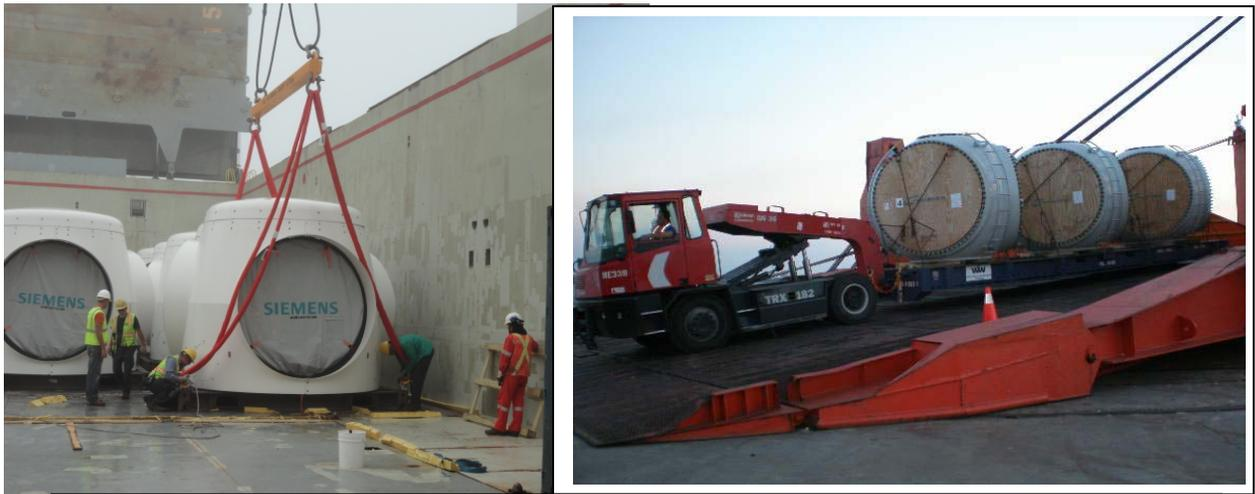
Rotors are transported as break bulk cargo and can be carried within ship's holds or transported on mafi trailers, aboard Ro-Ro ships.
